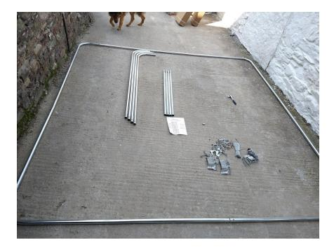
4: Attach uprights using clamps, bolts and nuts provided. Uprights are bar number 3
